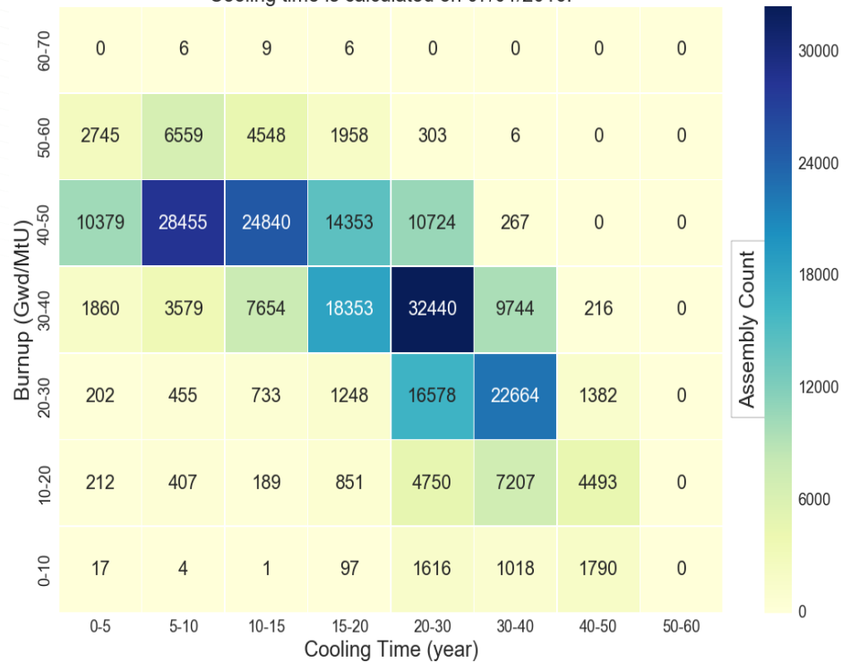
SNF inventory (discharged from US commercial reactor through June 2013) from the Unified Database binned by burnup and cooling time. Cooling time is calculated on 07/01/2016.
