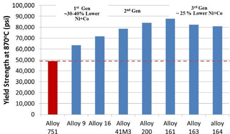
*Yield strengths of new alloys are up to 80% greater than that of alloy 751, which is currently used as a valve material.*
