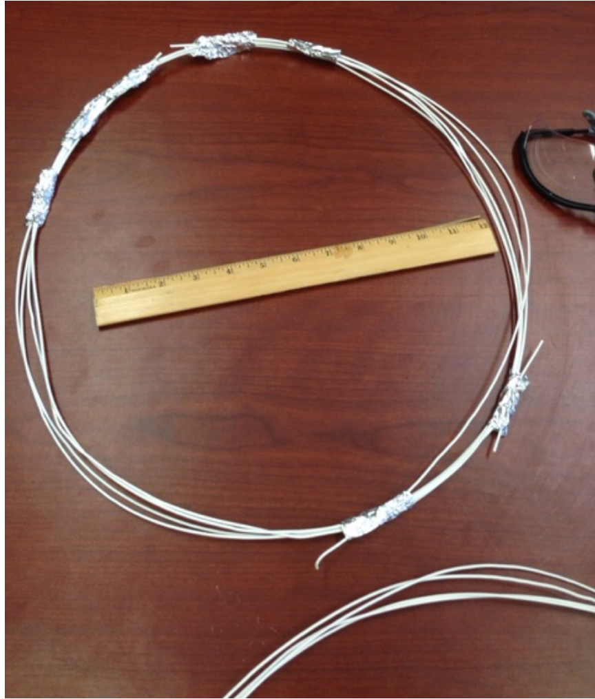
Fig. 4. Picture of extruded filaments with a 33.7% volume concentration of boron nitride particles, illustrating their flexibility.
