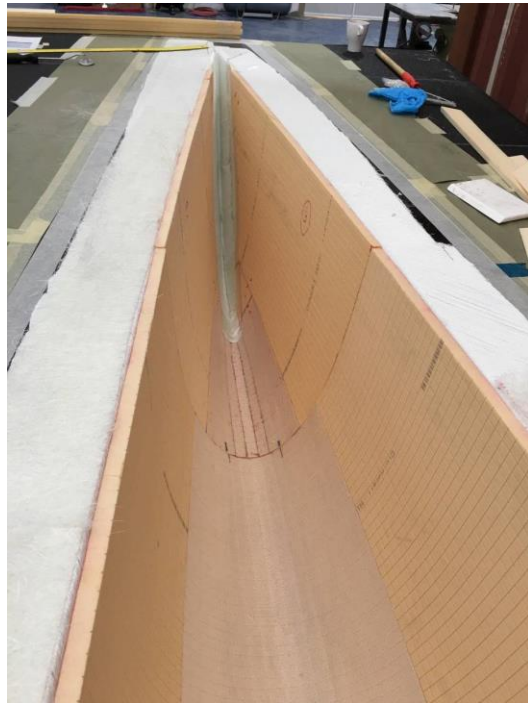
Figure 36: Placing a foam core into the mold.
