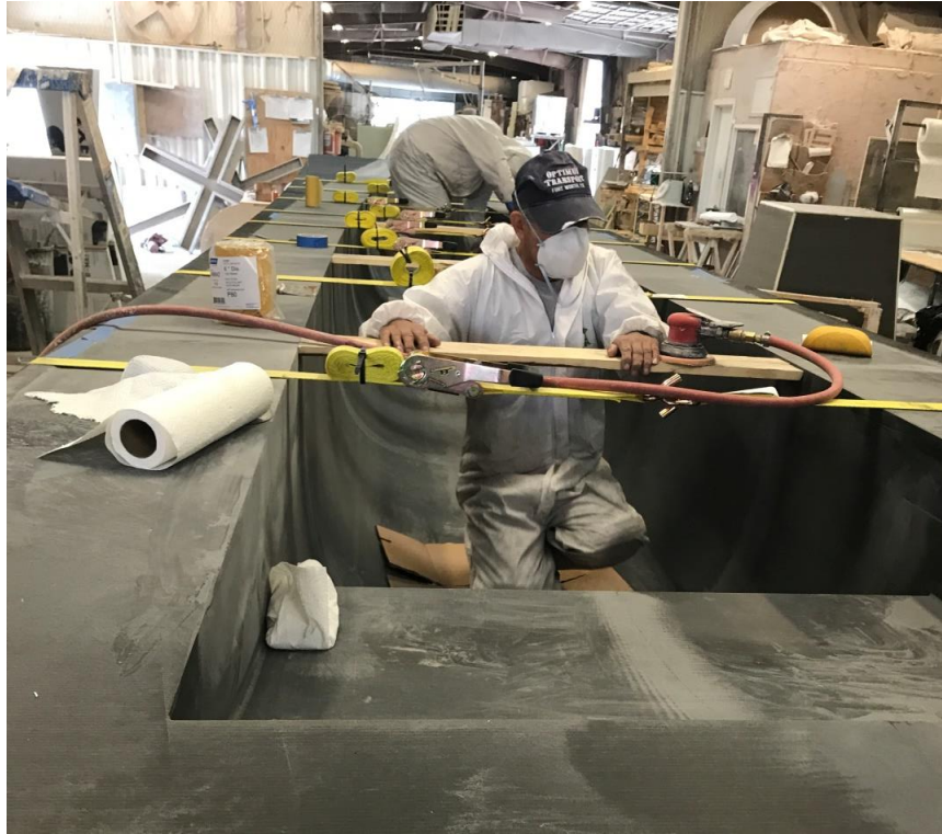
Figure 31: 320 grit surface finishing.
