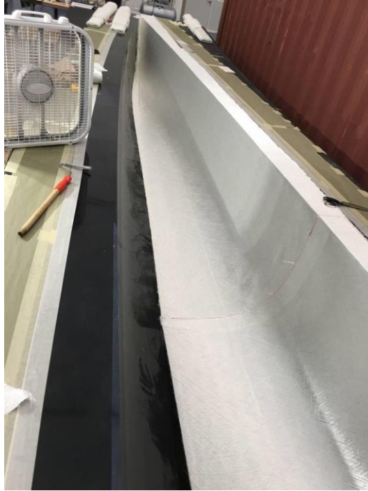
Figure 35: Laying up the mold with fiberglass fabric.
