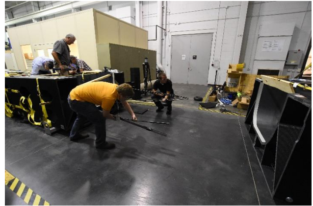
Figure 19: Guiding tensioning rods.
