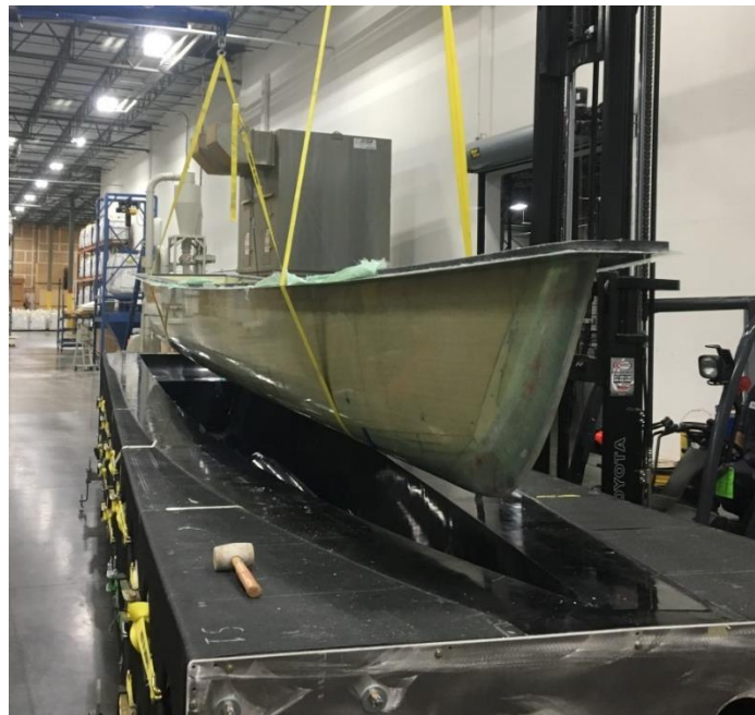
Figure 38: Cured infused hull from the mold.
