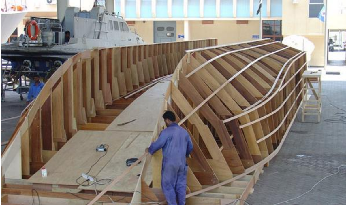
Figure 1: Traditional manufacturing of a plug.
