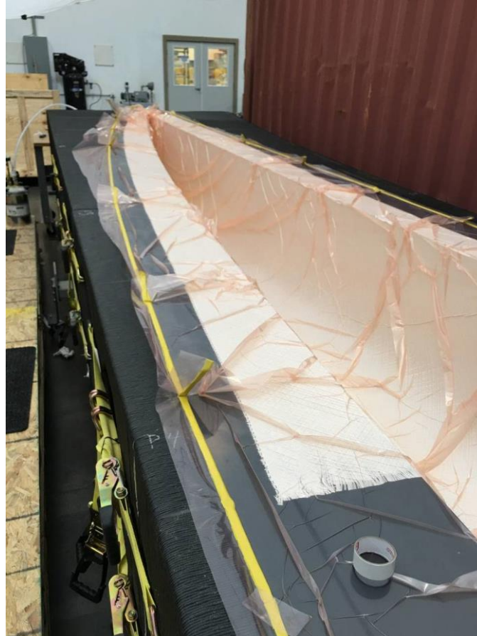
Figure 33: Mold under vacuum test.
