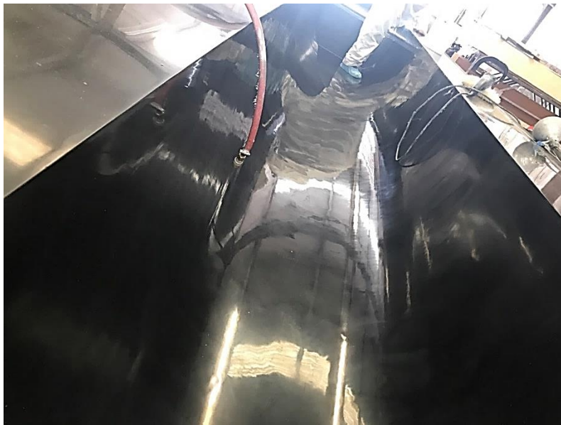
Figure 32: Mold coated with a vinylester mold surface agent.
