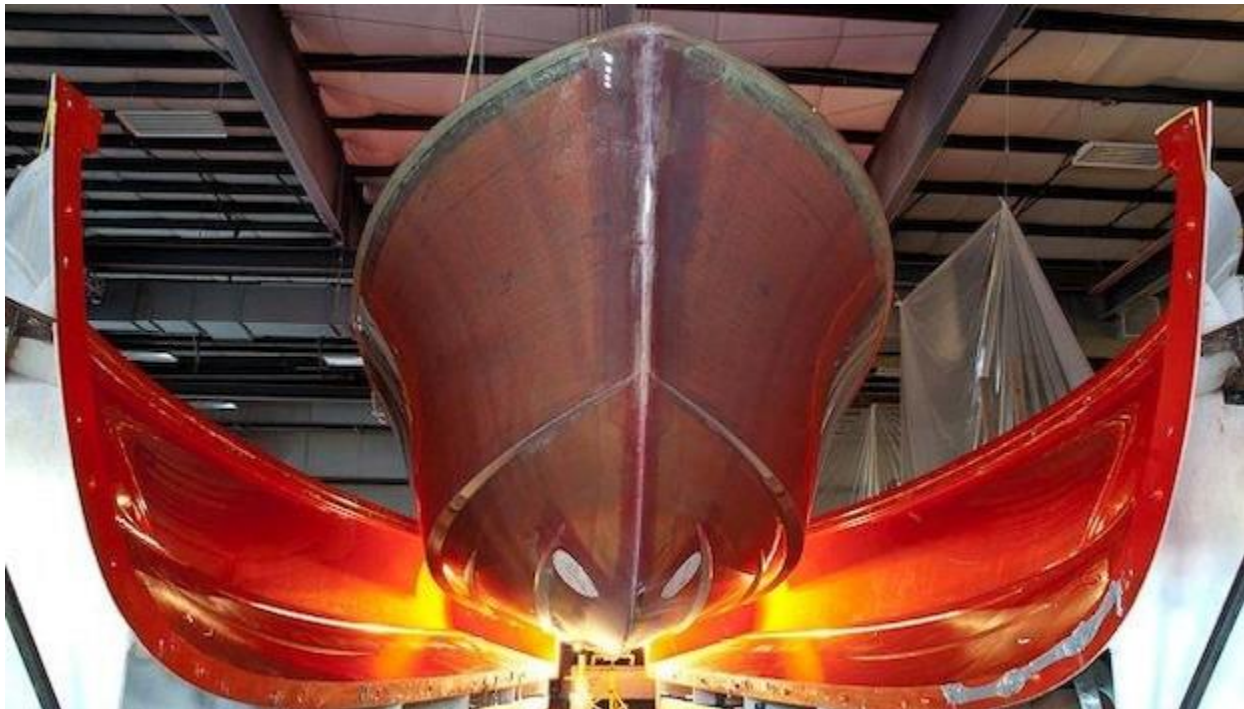
Figure 2: Molds manufactured from a plug.
