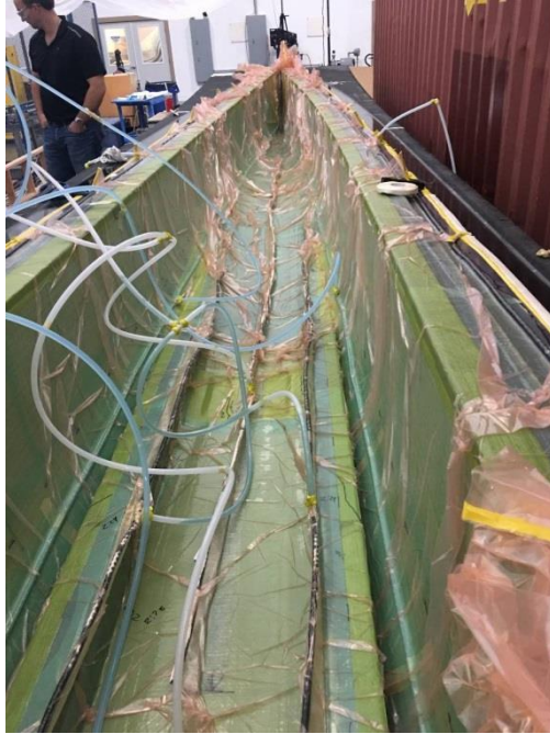
Figure 37: Infusing resin into the mold.
