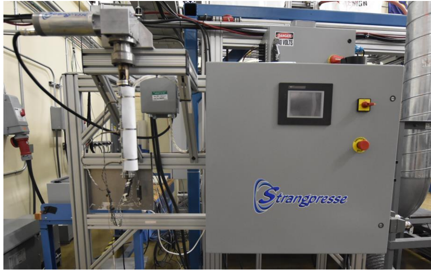
Fig. 3. The small Strangpresse extruder mounted on its testing apparatus with the extruder control box mounted beside the extruder.
