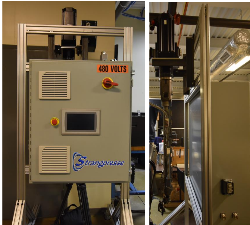
Fig. 4. The large extruder mounted on the back of its testing apparatus (right) and the extruder control box mounted to the front of the testing apparatus (left).
