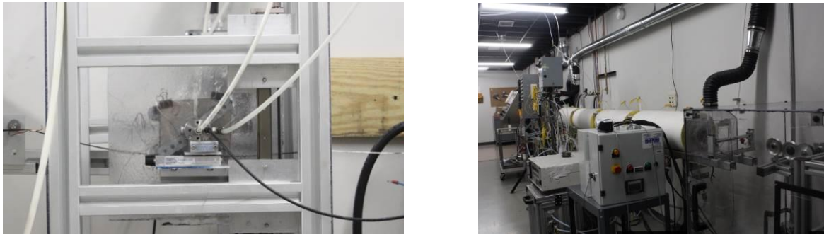
Figure 3: [Right] the spray sizing unit seen from the side. It can treat up to three tows at a time (only one is visible in this picture). The tows travel from left to right. [Left] The surface treatment is a long tubular unit with 4 heat zones.
