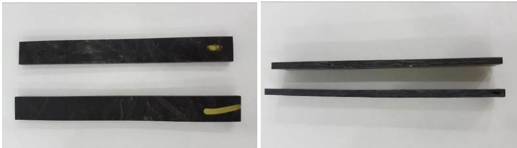
Figure 9: Both pictures show the same specimens, one from each panel, from front and side view (after mechanical tests). On the top, the “CONTROLw/IndSzg” specimen shows clearer tow strands from the front view (left) and more pores from the side view (right) than the specimen from the panel “SAMPLE”, shown in the bottom position on both pictures.
