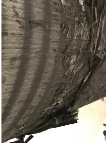
Figure 5: With the SMC process, the spray sized tows were undamaged and experienced clean cuts. However, they remained attracted on the surface of the final roller, preventing a normal release of the chopped material. This issue can be solved by changing the surface material of the line rollers.
