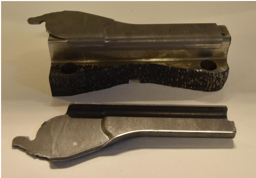
Fig. 2. DTS tool with stamped part attached to illustrate accurate fit.
