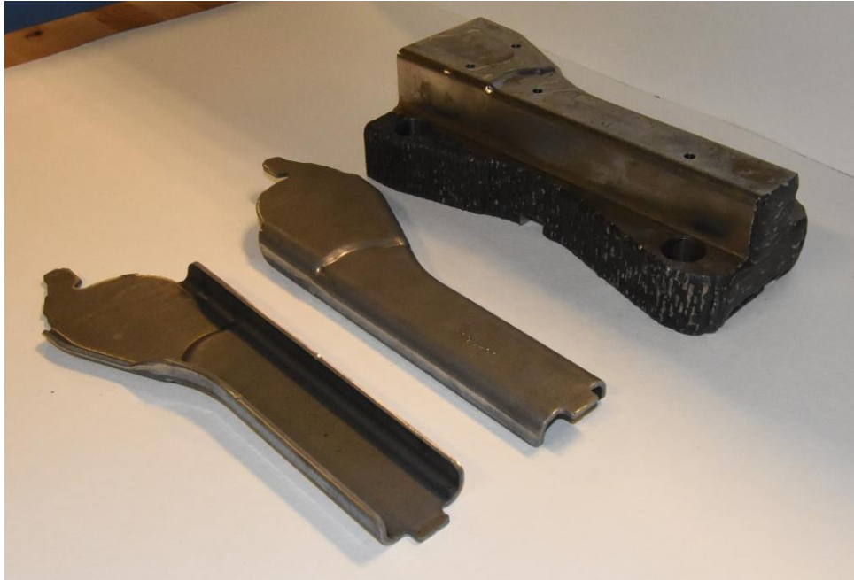
Fig. 1. DTS tool after machining (right) with stamped parts that were manufactured using the tool (left).
