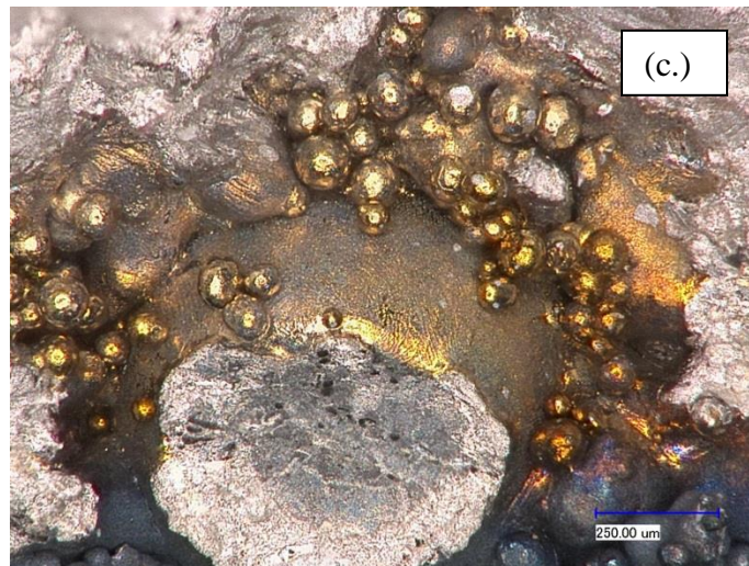
Figure 20. Optical images of sample V2 from batch 2 of 1/8 inch from (a) 30X, (b) 100X, and (c) 200X. These images show interconnected porosity that was open to the surface during HIP and heat treatment.
