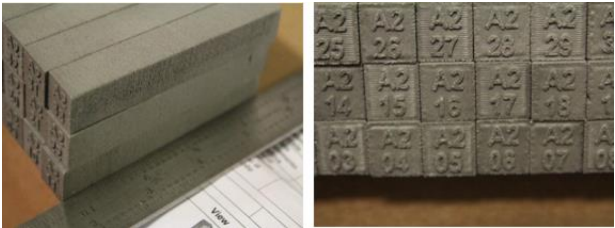
Figure 4. Horizontal LCF/tensile specimens built with EBM.
