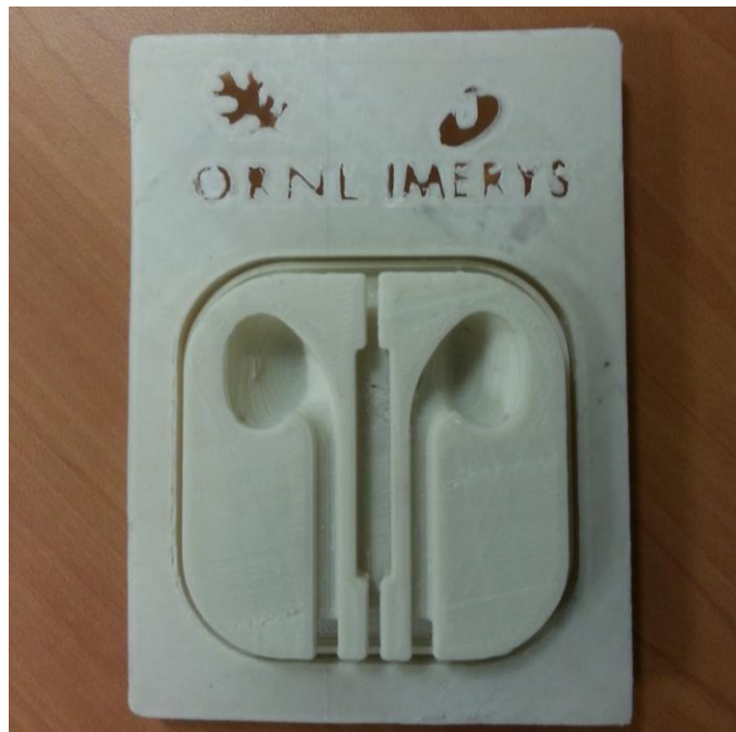
Fig. 3. Earbud case that was 3D-printed using 10% freeze-dried fiberlean and PLA.
