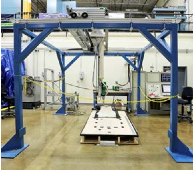
Fig. 1. Big Area Additive Manufacturing at the ORNL MDF.
