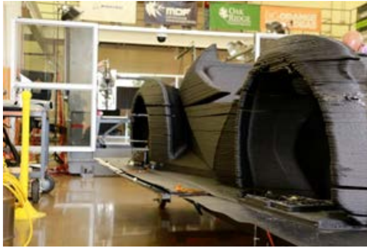
Fig. 9. Car 1, showing delamination.
