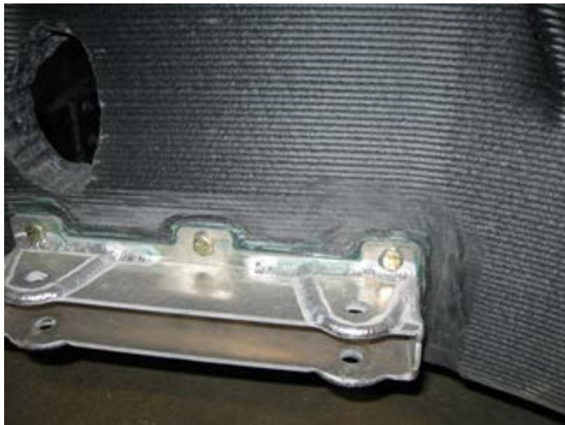
Fig. 8. Metallic bracket for integration of metallic components.
