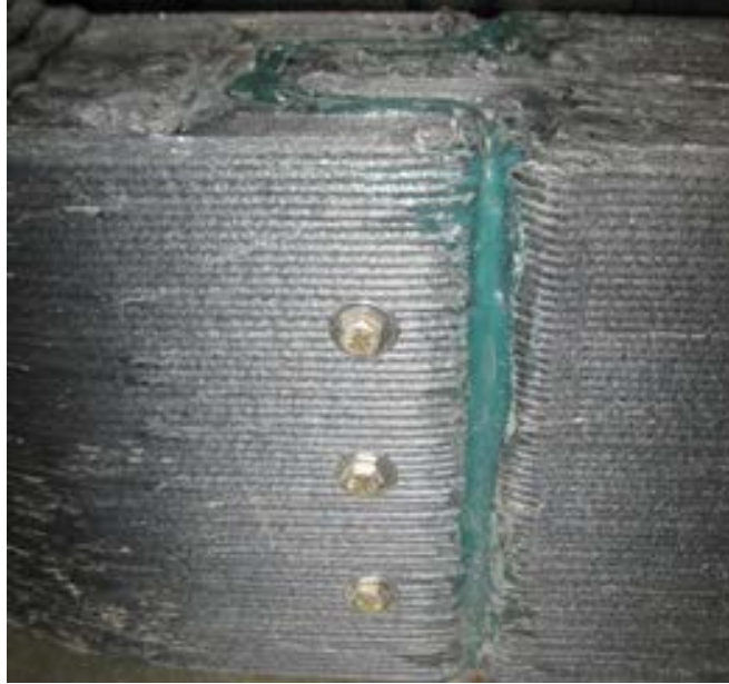
Fig. 7. Dovetail joint to join two composite parts.
