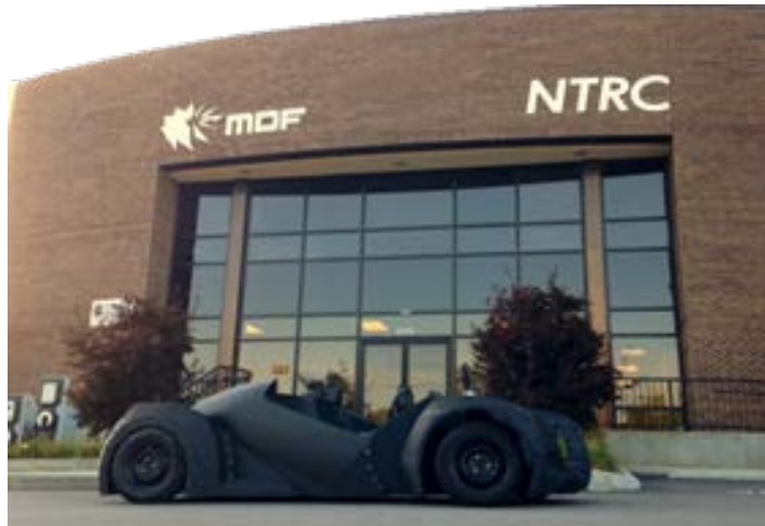
Fig. 10. Car 2, printed in four parts with no delamination.
