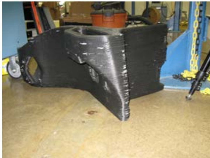
Fig. 5. Break away support for overhanging structures.
