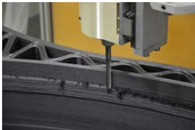
Fig. 3. Integrated machining head into the BAAM system.
