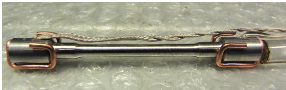
Figure 2 An example of the replacement rough machined, austenitized and quenched tensile couples used for the second series of HMFP parametric study experiments.
