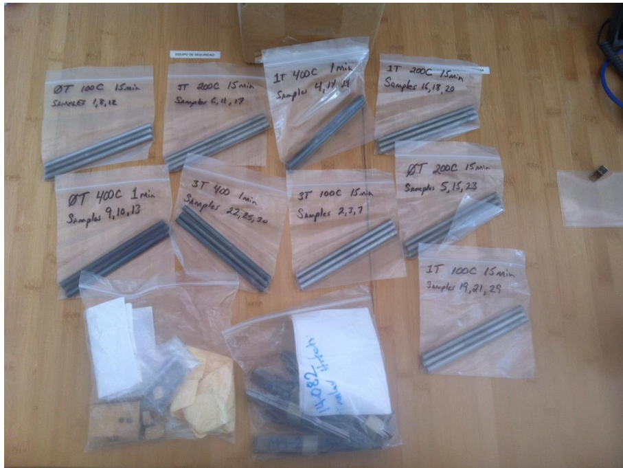
Figure 1 Part of the first series of HMFP samples that inadvertently did not get the prior austenitization and quench heat treatment at the industrial partner's facility before receiving the subsequent HMFP tempering treatment at ORNL.
