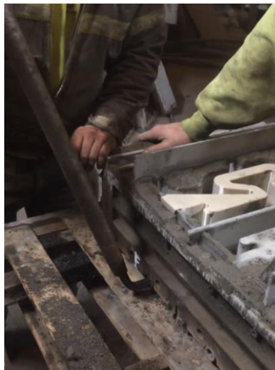
Fig. 3. Mounting the printed mold parts in a block production frame.
