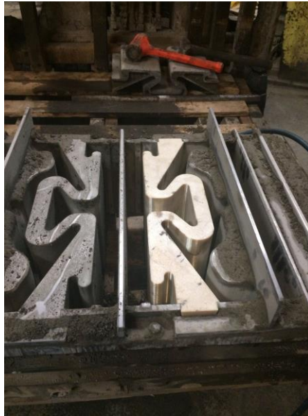
Fig. 4. Printed block molds (right) mounted alongside traditionally manufactured molds (left) in a block production frame.
