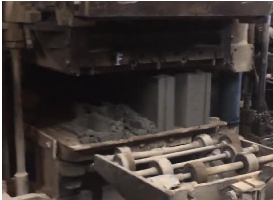
Fig. 5. Collapsed block from printed block molds (left) alongside traditionally manufactured block (right) on a block production line.
