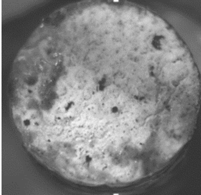
Fig. 6. Light microscope cross-section of a 1% CNT-ABS filament (diameter 1.7 mm) showing CNTs as dark spots.
