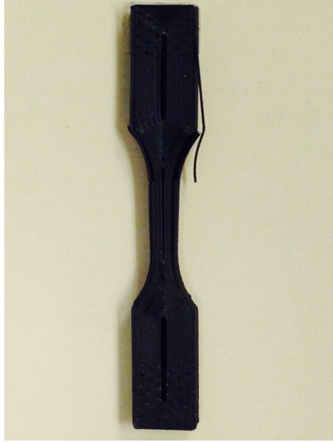
Fig. 11. Tensile bar (ABS with 1wt. % CNTs.) This bar was not tested due to its poor quality.
