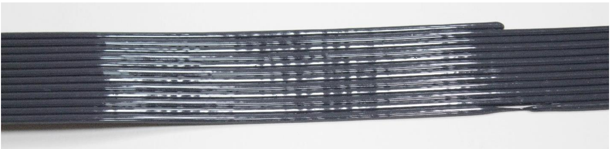
Figure 19: Close-up of high-speed raster showing individual beads
