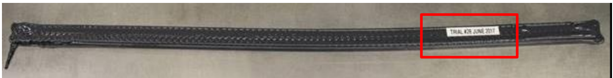
Figure 14: Curl bar showing a lack of deformation from thermal stresses. In the case of a thermoplastic material this bar would show warping from thermal stresses built up during deposition
