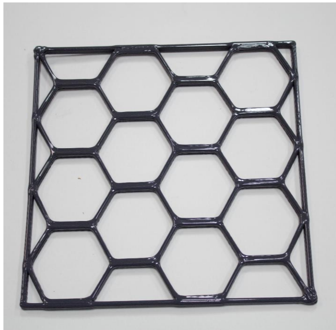
Figure 16: Honeycomb build showing the ability to build single bead walls
