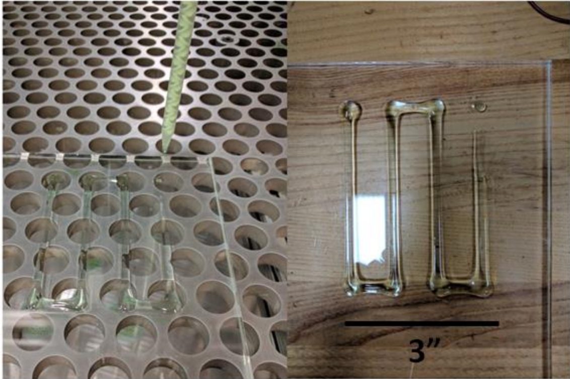
Figure 8: Test path printed using alcohol based non-reacting surrogate material. The spreading shown is due to the lack of gel strength.
