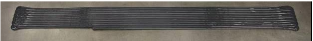
Figure 18: High-speed raster pattern printed at a rate of 300mL/min with a move speed of 9” per second
