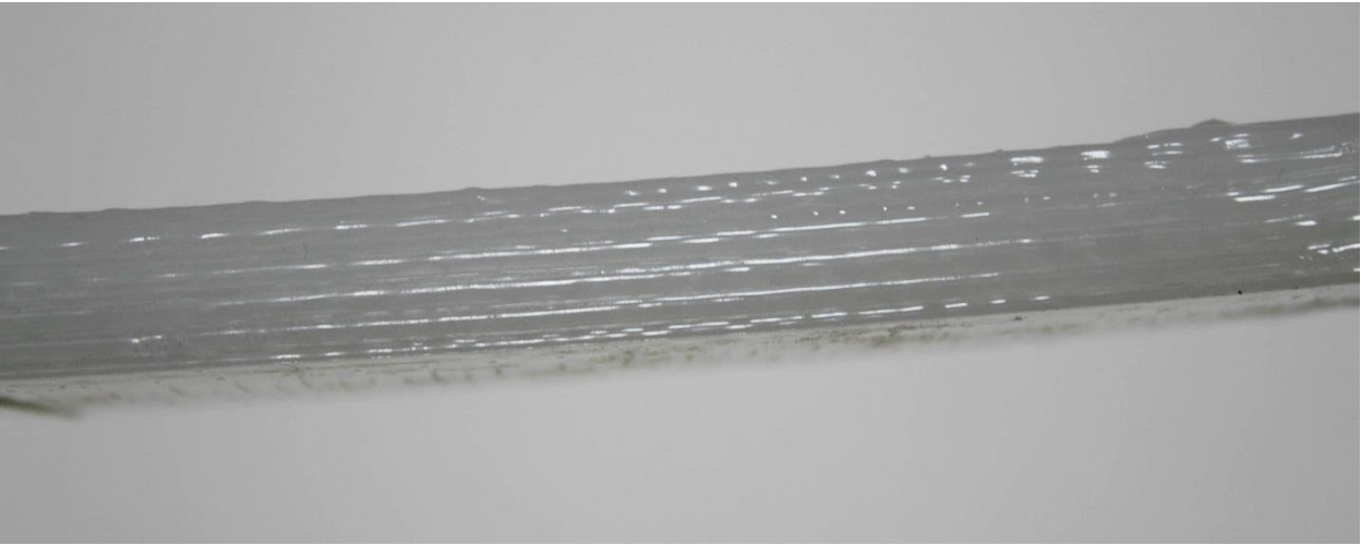
Figure 12: Large scale test bar edge showing good layering on border
