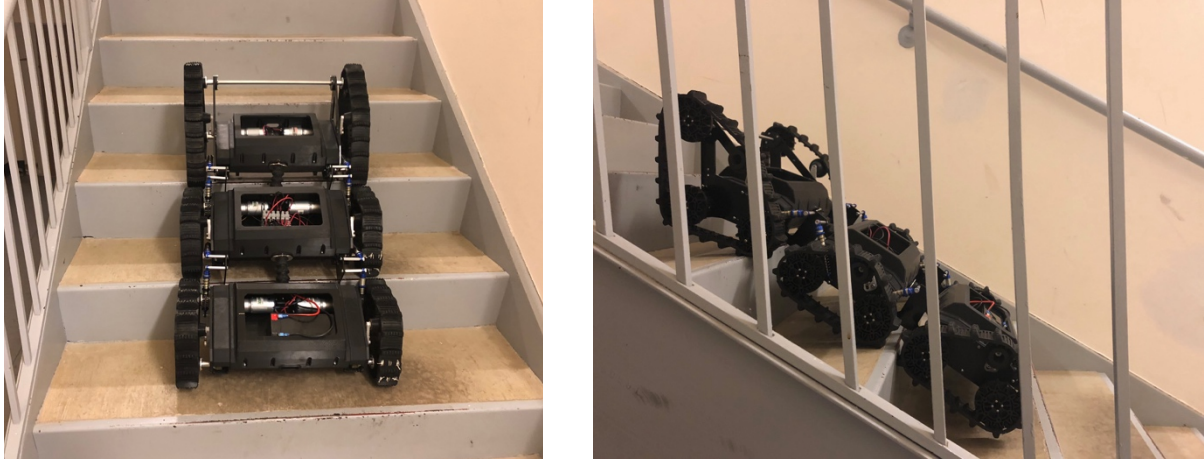
Fig. 4 Assembled ARTI climbing stairs
