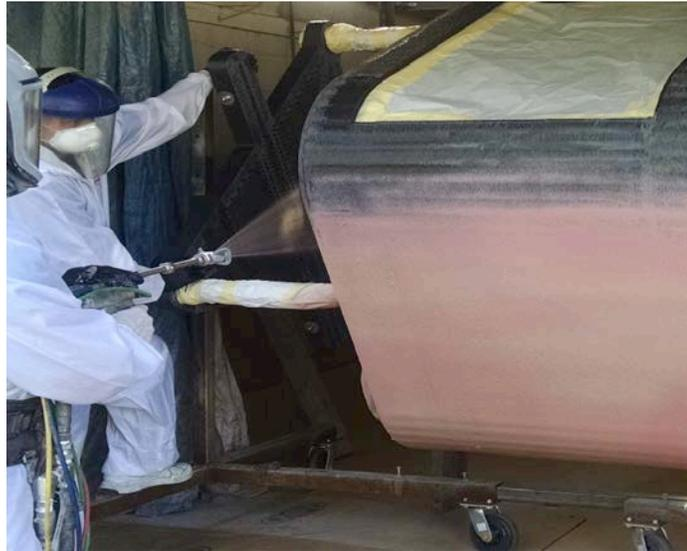
**Fig. 6. Spray application of *TD Coat RT* onto a vertical face of a printed surface.**
