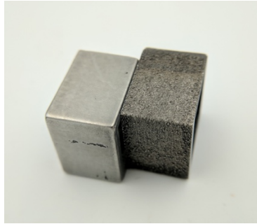
Figure 3: Comparison of cube artifacts showing the ability to enhance the surfaces to 1 \mu\text{m} Ra. The post-processed surfaces are shown on the left and initial surfaces on the right.
