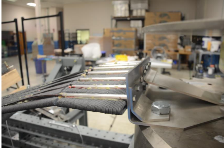
Fig. 6. Test set up using root bushings and bolts.
