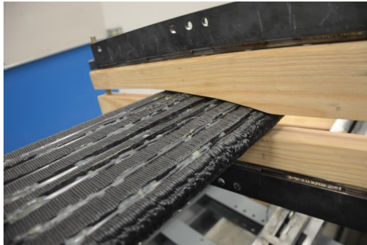
Fig. 7. Carbon fiber rods inserted and glued into the cut grooves of a prototype blade.
