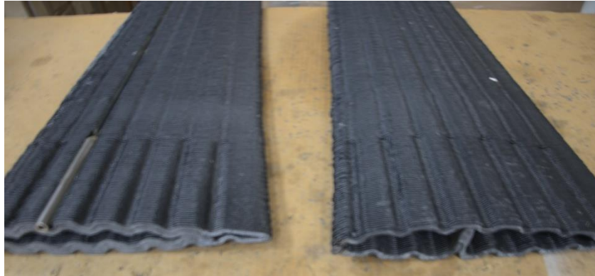
Fig. 4. Prototype blade with two bead thick walls with a spar sitting in a groove (left) and a second prototype blade with a single bead wall and no spar (right).
