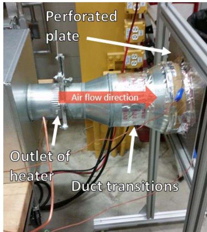
Figure 10. Test stand for shakedown testing of different duct diameters with perforated plate
