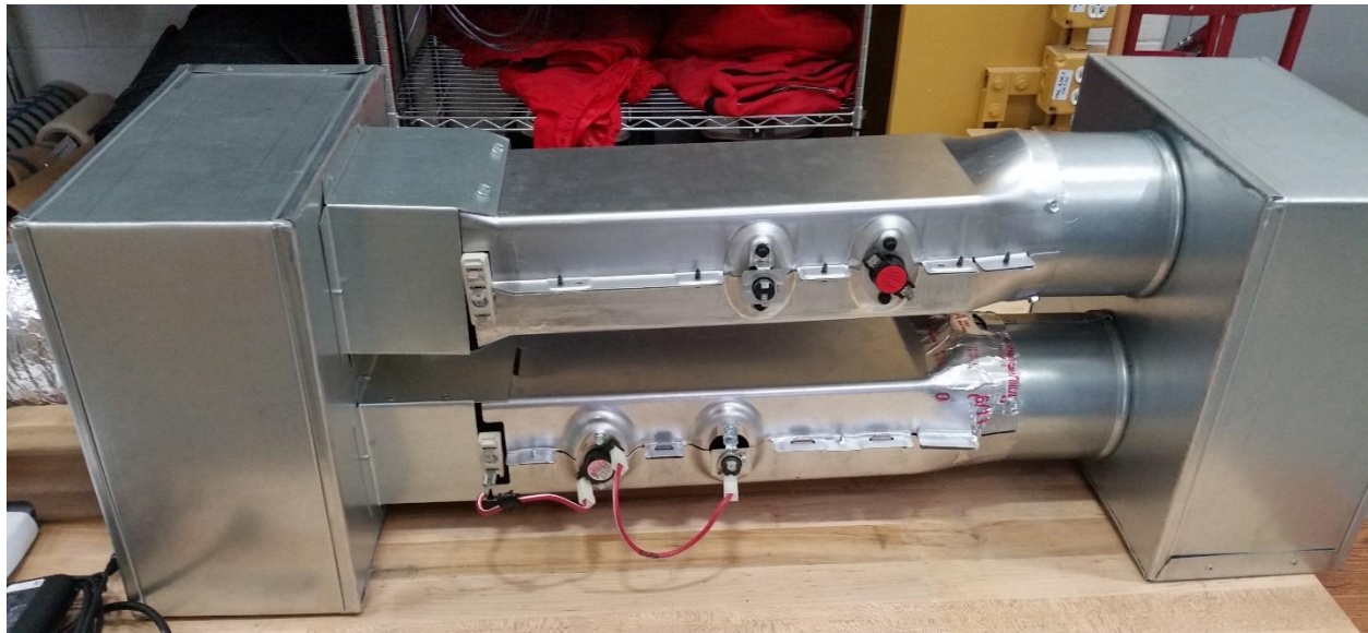
Figure 4. Completed heater assembly showing inlet and outlet plenums (air flow from left to right)
