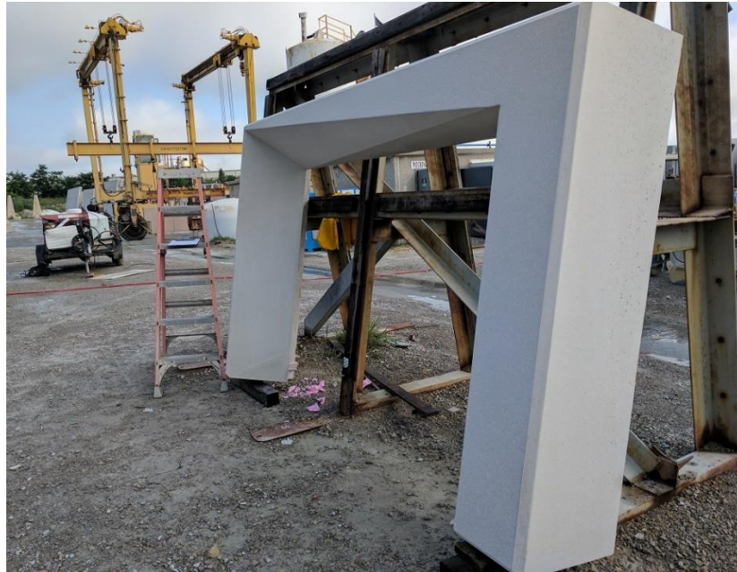
Figure 1. Precast mockup that was produced using a 3D printed mold from Phase 1
