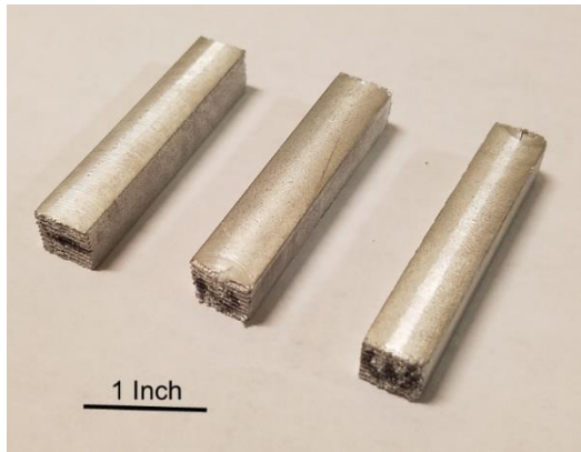
Figure 3: Bend bars (after machining).
