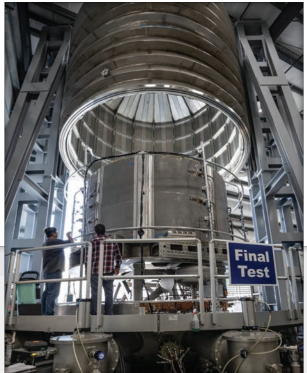
The magnet module in the final testing chamber. Image credit: General Atomics
