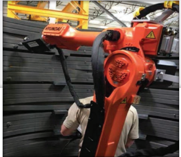
An ultrasonic peening robot strengthened critical welds in the coil. Image credit: US ITER
