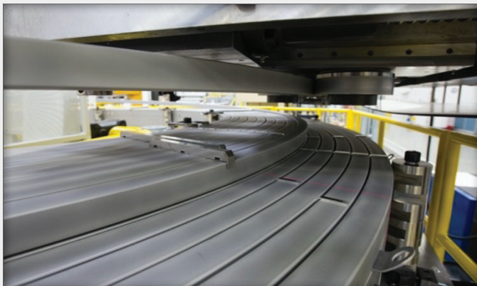
Precision winding of conductor. Image credit: General Atomics
