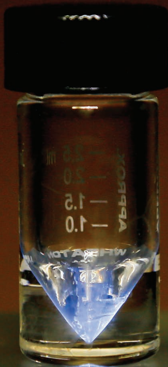
This irradiated sample of Ac-225 at ORNL’s Radiochemical Engineering Development Center glows blue because of the ionization of surrounding air by alpha particles. Earlier this year, the FDA received the drug master file for Ac-225 nitrate produced at ORNL from a thorium-229 stockpile. The isotope is in demand because it’s an ingredient in targeted cancer treatments. Image credit: Jason Richards, ORNL
