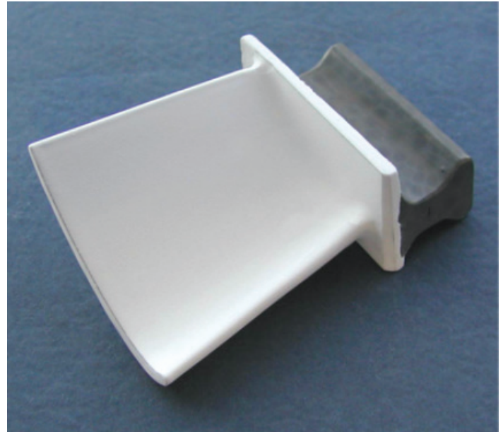
Fig. 2. Example of a rare earth-doped silicate coating on a \text{Si}_3\text{N}_4 vane. [Credit: B. L. Armstrong]
