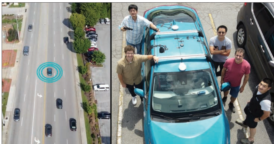
ORNL researchers took a connected and automated vehicle out of the virtual proving ground and onto a public road to determine energy savings when it is operated under predictive control strategies. Image credit: ORNL
