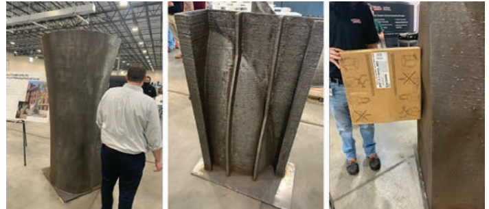
Figure 2. Additively printed large-scale parts of ~5–10 ft. (Credit: Lincoln Electric).
