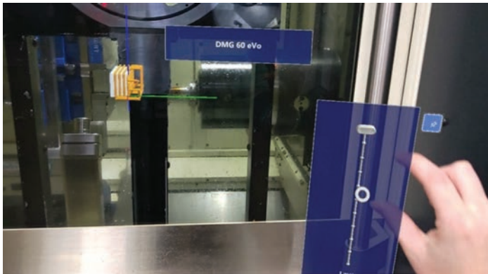
Figure 4. Example visualization of SAMARAI view. The stock to be machined is represented as the white block, and the yellow segments surrounding it represent the G-code pathing. (Credit: Borish, ORNL).
