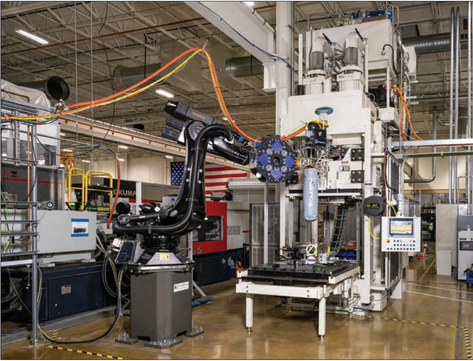
ORNL's additive manufacturing compression molding, or AMCM, technology can produce composite-based, lightweight finished parts for airplanes, drones or vehicles in minutes. Image credit: Carlos Jones, ORNL
