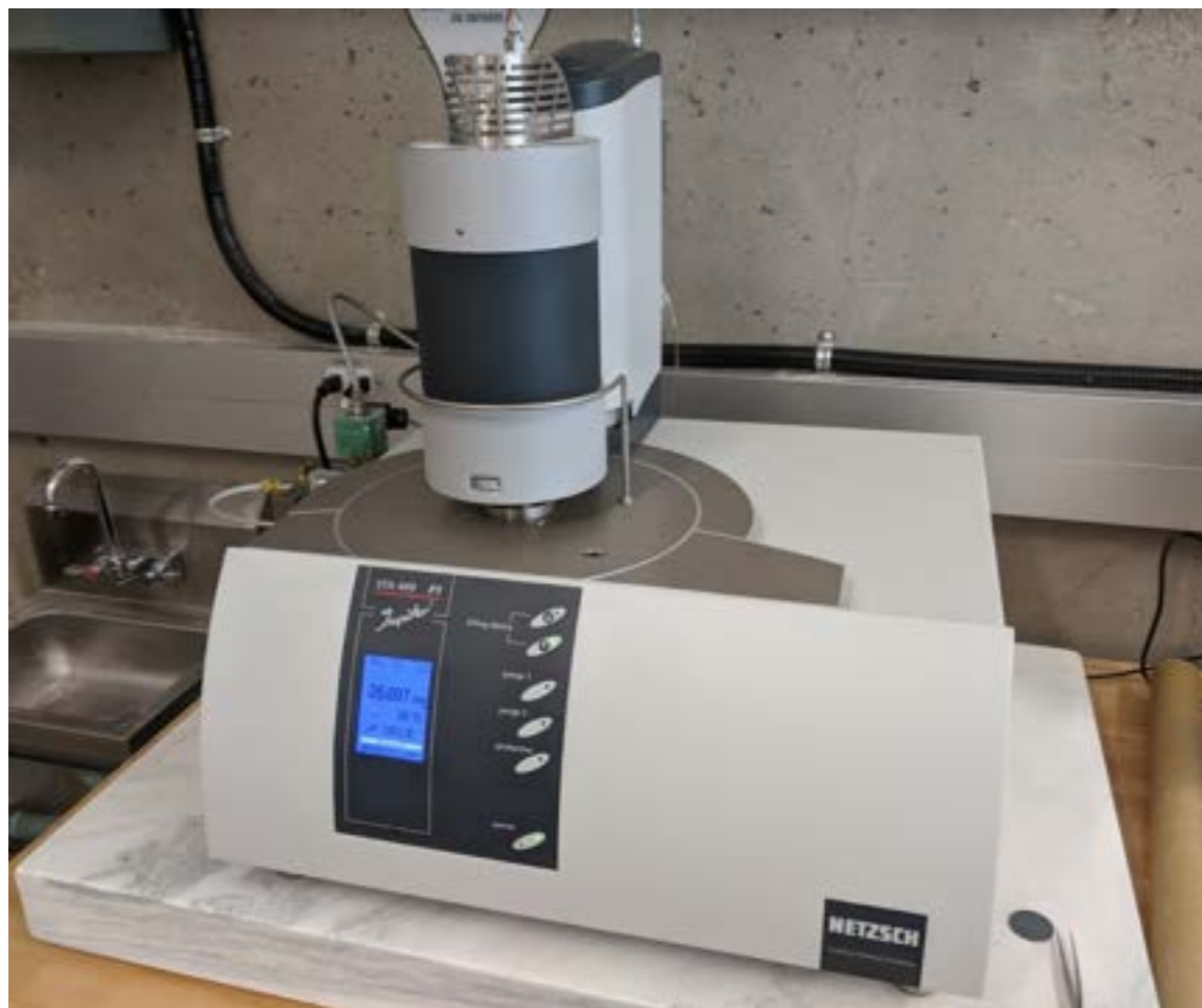
Netzsch Jupiter STA 449 F1: DSC + TGA for thermodynamic measurements on salts
