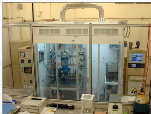
Computer-controlled fluidized-bed CVD coating system
