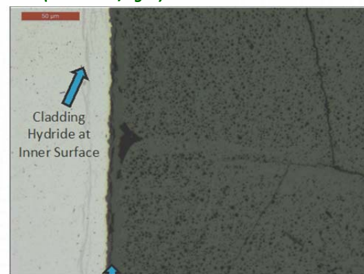
Rim Structure in High Burnup Commercial LWR Fuel (~70 MWd/kg U)
