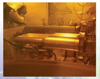
Figure 42. SNS mercury target.
