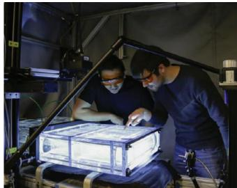
*Figure 36. Flow visualization and application of PIV and PLIF to measure velocity distributions inside an SNS target*
