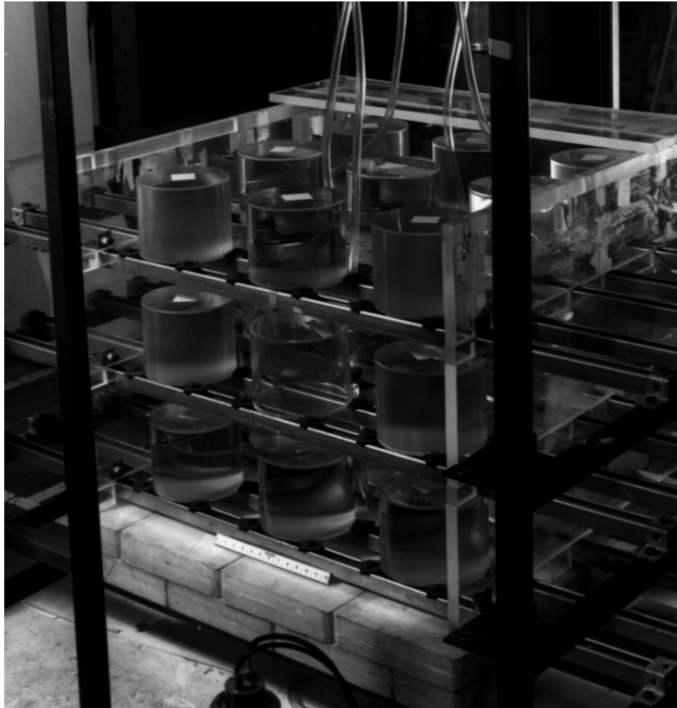
Figure 8.1.C.8. View of a 27-unit array with 2.54-cm. thick Plexiglas reflector on five sides and a 15.24-cm. thick paraffin base.
