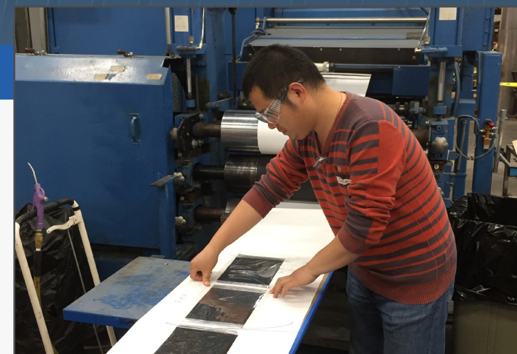
ORNL’s Zhijia Du prepares material samples for electron beam curing, which instantly cross-links the binding resins in coating material at a high line speed of 500 feet per minute.
