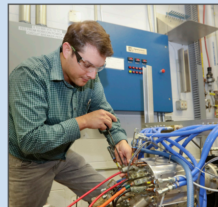
Researcher Tim Burress works with a prototype motor that uses ferrite permanent magnets.
