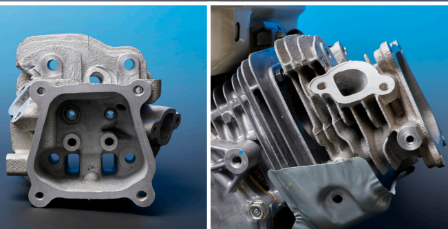
The aluminum–cerium alloy does not require heat treatment and maintains 100% of room temperature mechanical properties after 1,000 hours at 400°C.
