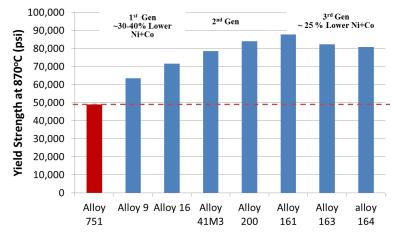
Yield strengths of new alloys are up to 80% greater than that of alloy 751, which is currently used as a valve material.
