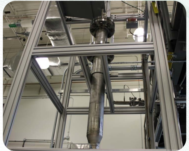
Condenser Section of the Thermosyphon Test Loop
