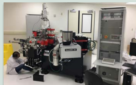
Left: Class 100 (ISO 5) metal-free clean room for trace uranium and plutonium chemistry and preparation; Center: Researcher operating thermal ionization mass spectrometer in the mass spectrometry wing; Right: Installation of a new CAMECA® NanoSIMS 50L in the NanoSIMS Suite.
