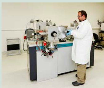
Left: Class 100 (ISO 5) metal-free clean room for trace uranium and plutonium chemistry and preparation; Center: Researcher operating thermal ionization mass spectrometer in the mass spectrometry wing; Right: Installation of a new CAMECA® NanoSIMS 50L in the NanoSIMS Suite.
