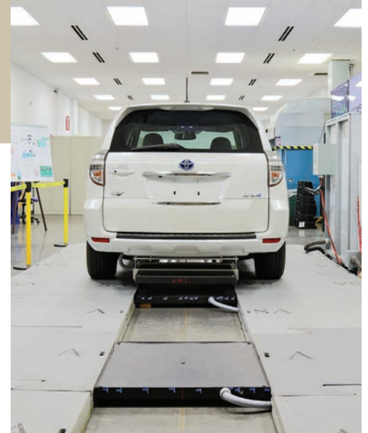
ORNL's 20-kilowatt wireless charging system features 90 percent efficiency. (Photo by Jason Richards)
